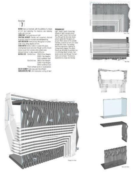
Figure 5. TOGS3 (Temporary Outdoor Gallery) Finalist Competition Submittal using duct work to create auditory connections through the walls of the installation.
